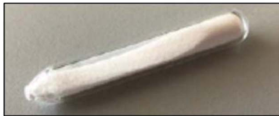
Figure 1: Target Ampule – Cylindrical fused quartz body containing target material
